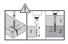
CAUTION: These boards should be pre-drilled and countersunk to avoid cracking. *Adjust countersink tool to width of first board to countersink to proper depth. Pre-drill into second board using first board as a template before attaching.*
