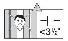
CAUTION: Spacing between boards must be less than 3<sup>1</sup>/<sub>2</sub>" (or greater than 9") or a head/ neck entrapment could exist.
