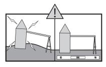
CAUTION: Ground must be level. Installation on a hill or incline will create unsafe conditions.
